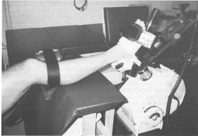
Figure 1 — Positioning of subject on the Kin-Com II isokinetic dynamometer for ankle joint position sense testing.
